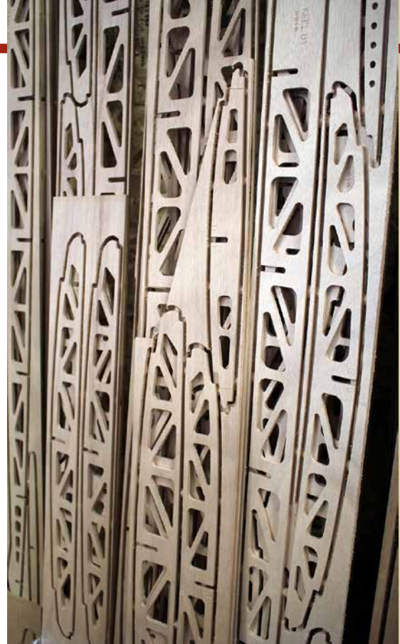
Marine plywood is used for the internal portions of the boards. These parts are cut on a CNC (computerized numerical control) machine and are based directly on the computer model of each shape.
