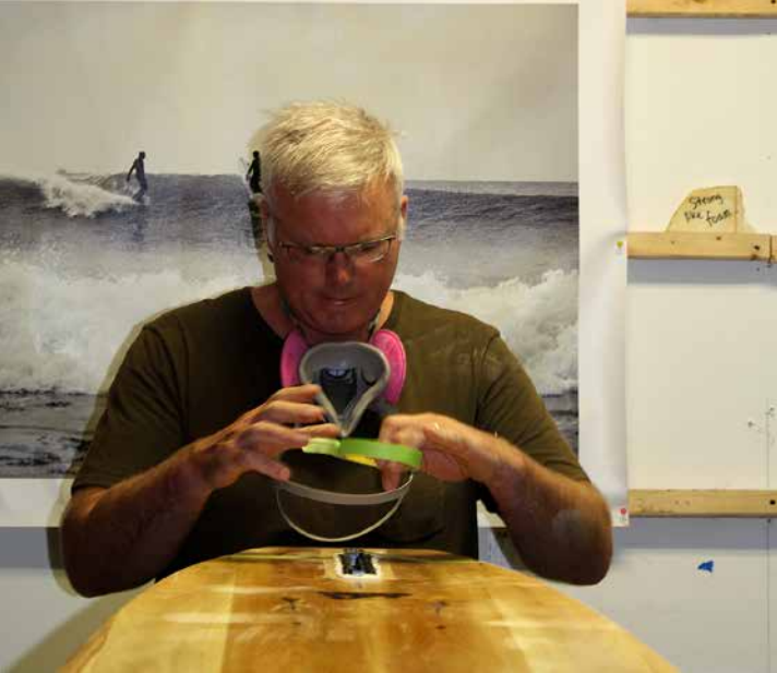
John H. tapes a fin box into place while a resin hardens.
