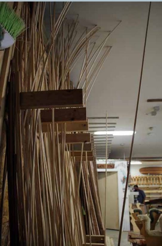
Thin “bead and cove” strips are used to build up the rails during construction of the surfboards.
