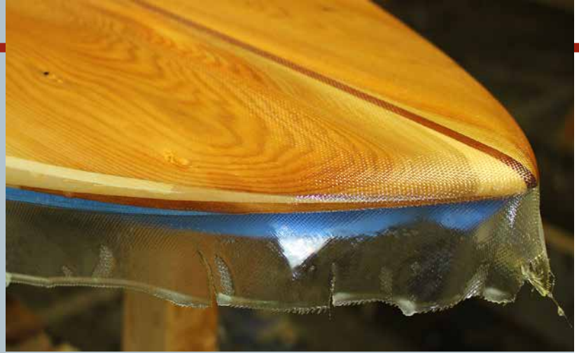
Closeup of the rail of a wooden surfboard during an early stage in the fiberglass process.
